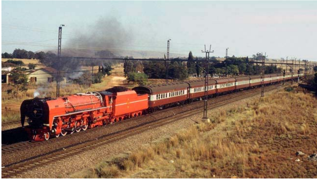
A) South African Railways Class 26 4-8-4 'L.D.Porta'. 'Porta Treatment' was an essential part of the modernisation scheme undertaken on this locomotive. It was also used elsewhere on the SAR 3'6" gauge network. © Roger Griffiths
