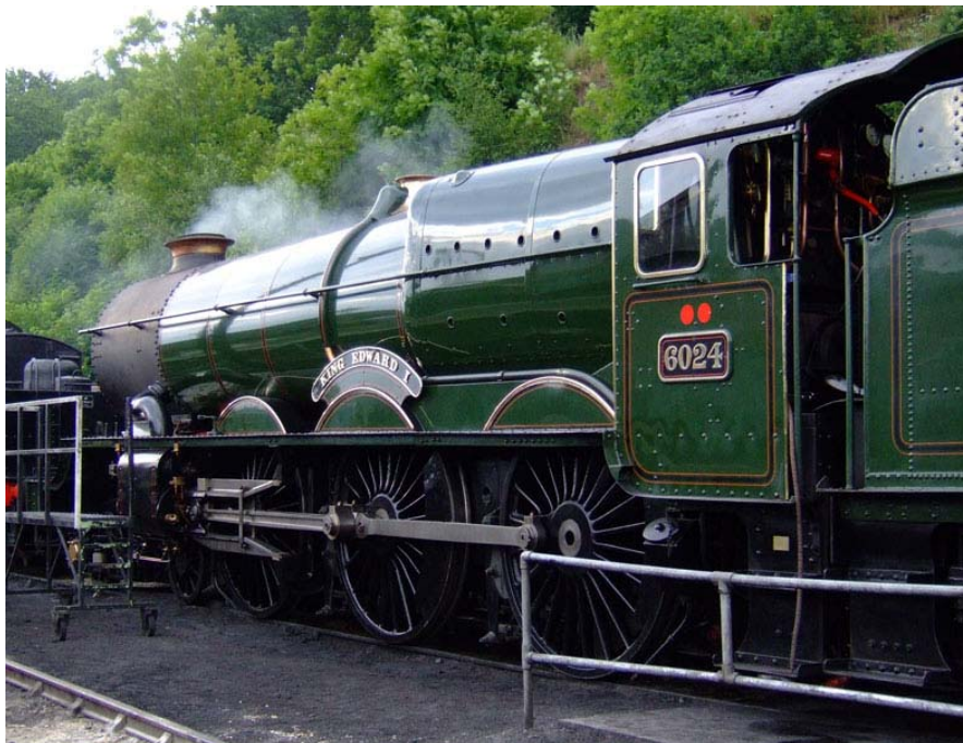
B) 6024 King Edward I, the first standard gauge locomotive outside of the Americas to use 'Porta Treatment'. (4)
